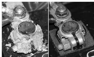
Corrosion build-up on a battery terminal
